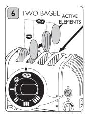
4 slot model: Rotate the 'selector switch' anti-clock-wise to the two bagel symbol. Only the second and forth element from the left will heat up.
